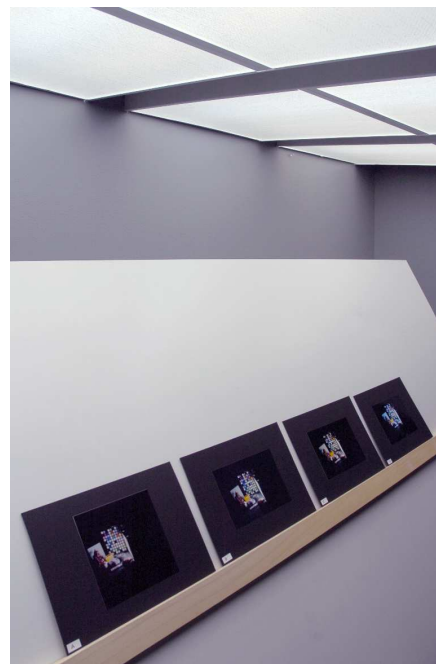
Figure 2. Experimental setup for printed image evaluation. The dedicated print viewing room includes ISO standard daylight illumination and gloss-free viewing arrangement.
