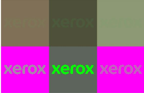
**Figure 10.** Ink pairs under the LED illumination according to the weights  $w$  in Fig. 8: top – no matrixing; bottom – optimized matrix  $M$ .
