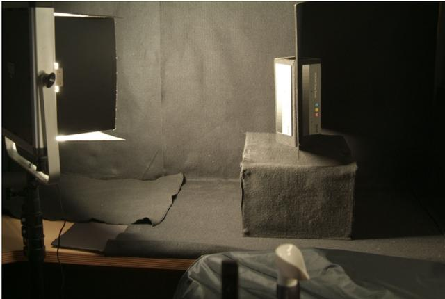
**Figure 2.** The lighting configuration used in this experiment. The cool-white florescent light set on the left side provides much higher illumination than the one on the far right side (not seen on the right).
