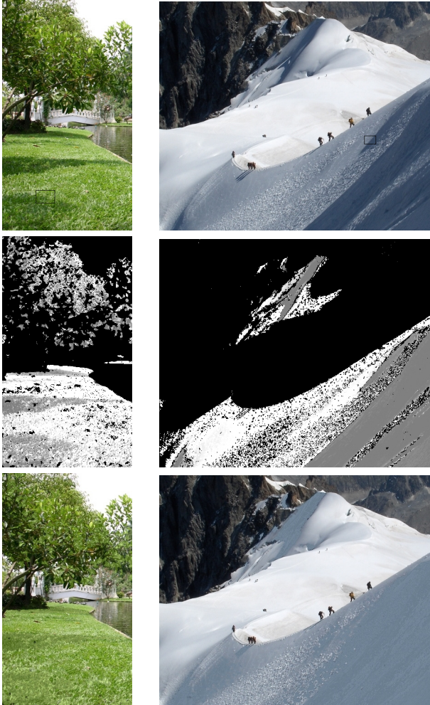
Figure 4. Shadow removal examples. Top: the original images. Middle: the detection maps. Bottom: reconstructed images with shadows removed using the proposed approach.
