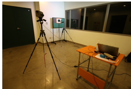
Figure 10. Setup for measuring viewing angle-dependent color shift under daylight.
