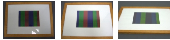
Figure 2. Viewing angle-dependent color shift of ChLCD. As the viewing angle increases, red shifts to green, green shifts to blue, and blue shifts to black.
