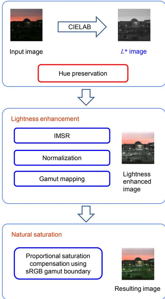
Figure 3. Procedure of the proposed tone reproduction method.
