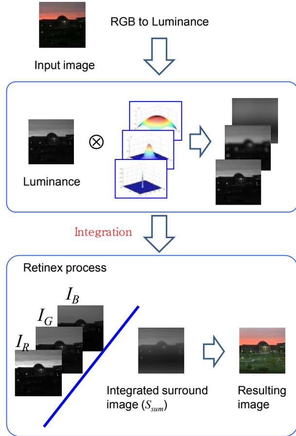
Figure 1. Flowchart for IMSR using integrated surround.
