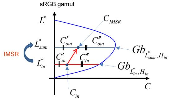
Figure 7. Saturation compensation.
