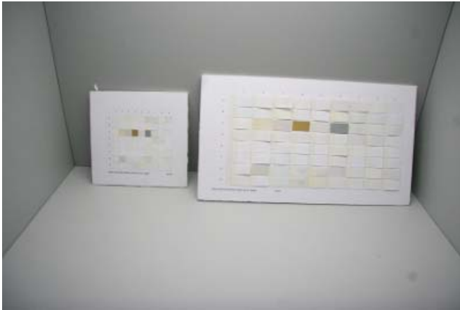
Fig. 3. Visual target, left, and tactile target, right, in the viewing booth. The visual samples were 15 mm square and the tactile samples were 35 × 20 mm and were attached by their left edge to the foam core base.
