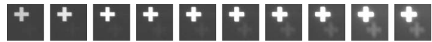
Figure 5. Exposure series of acquired images for high dynamic range imaging (500 nm band). It can be seen that the original cross symbol is acquired correctly as well as its weak ghosting duplicate.
