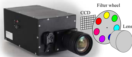
Figure 1. Seven channel multispectral camera with its internal configuration sketched.
