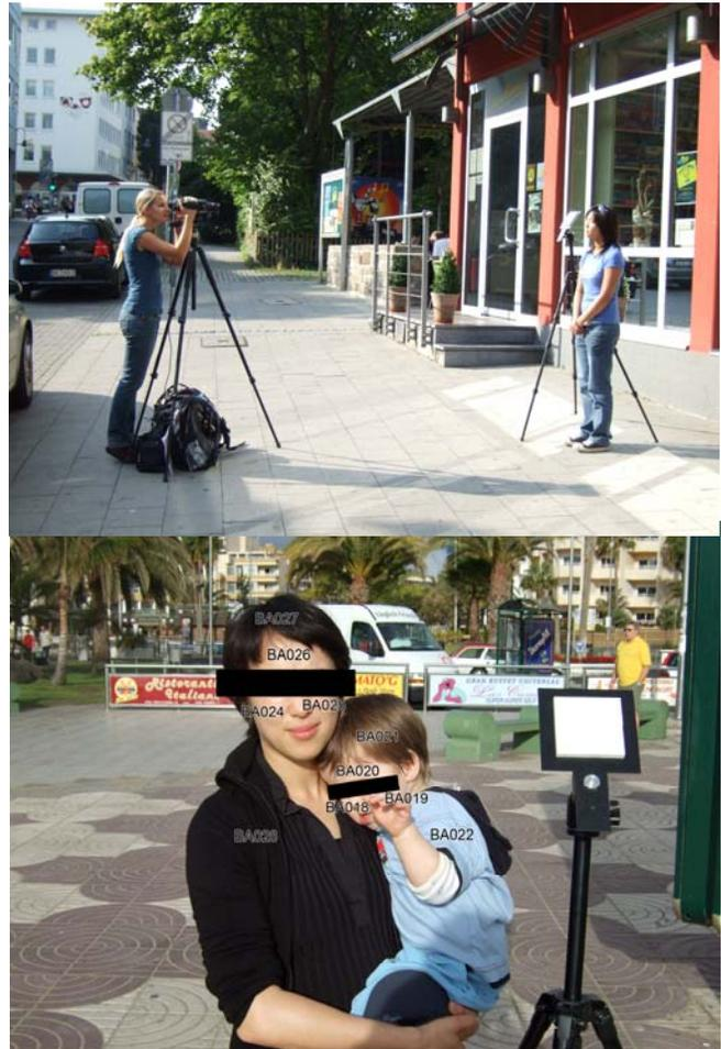
Figure 1: The upper image shows a typical measurement setup to measure skin tones and the lower picture shows a an example for the presentation of the results.
