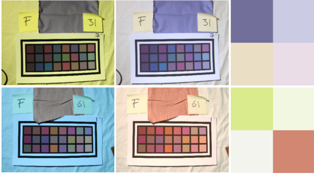
Figure 4. Paint samples are grouped in palettes of four colors. The system matches the object color to one of the paints and returns the corresponding palette. The figure shows, from left to right, the uncorrected image, the corrected image, and the corresponding paint palette.
