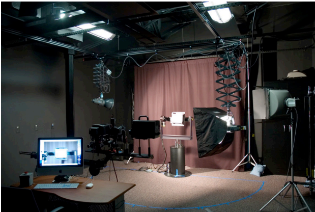
Figure 4. The gonio-imaging room. In the foreground is the computer used to control the entire imaging process along with the detectors. The lights are positionable from a grid on the ceiling. The three-axis sample positioner is visible in the center of the image.
