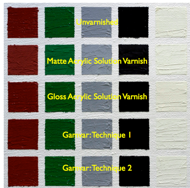
Figure 2. Acrylic paint on coarse canvas with a different type of varnish in each row. The paint was applied with a palette knife to create impasto.
