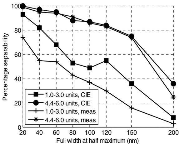
**Figure 9.** Results of the optimised sensor with 10-bits quantisation showing the effect of changing the illuminant on the separability results of the floral samples.
