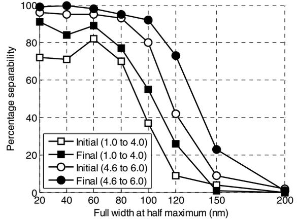
Figure 5. The separability results with both the initial and optimised sensor combinations when the sensor responses are quantised to 10 bits. (Tested with Munsell and CIE test daylight spectra)
