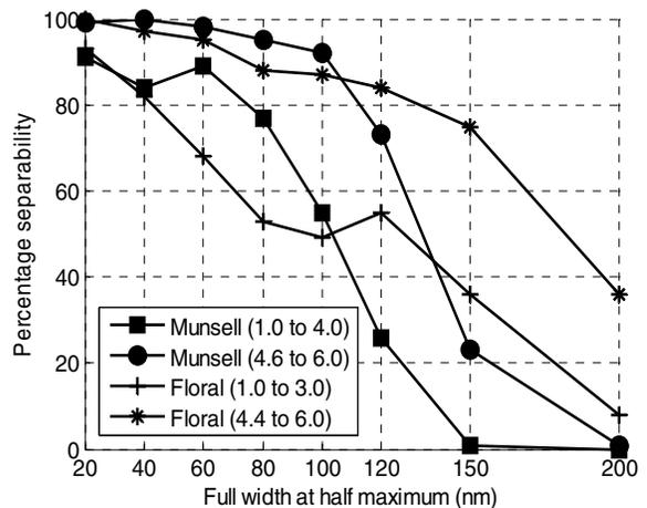
Figure 7. Separability results of the optimised sensor set with 10-bits quantised response. CIE standard test daylight was applied in this test.
