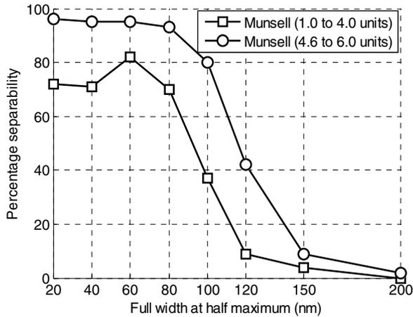
**Figure 2.** The separability results for the initial sensor combinations when the sensor responses are quantised to 10 bits. (Tested with Munsell and CIE daylight)
