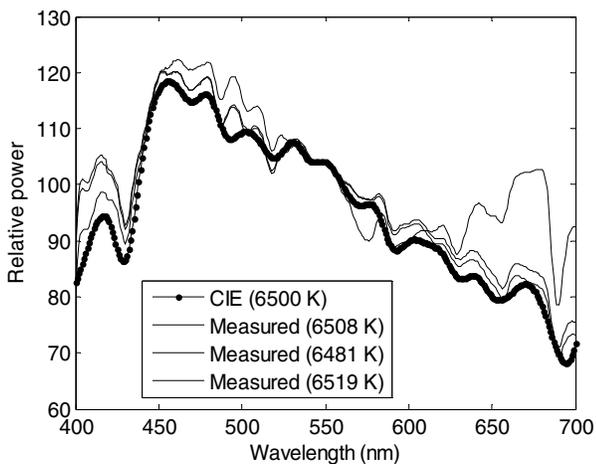
**Figure 10.** Spectra of CIE (6500 K) and measured daylight with correlated colour temperature 6508 K, 6481 K and 6519 K.
