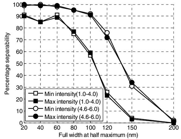
Figure 6. The colour separability results when the sensor responses are quantised to 10 bits for two illuminant intensities that differ by a factor of 120dB (or  $10^6$ ). This result shows that as expected this approach is able to deal with a wide dynamic range of inputs.
