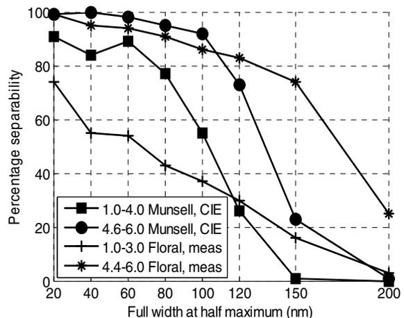
**Figure 11.** The separability results for optimised sensor combinations with 10-bits quantised response. The results shown are for the Munsell and CIE standard test daylights and floral with measured daylights which might represent data from a possible application.
