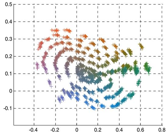
**Figure 4.** The two dimensional feature space formed by 80nm wide sensors from 202 Munsell surfaces and 14-CIE standard daylights after the sensor positions have been optimised. The data was quantised with 10-bits quantiser.
