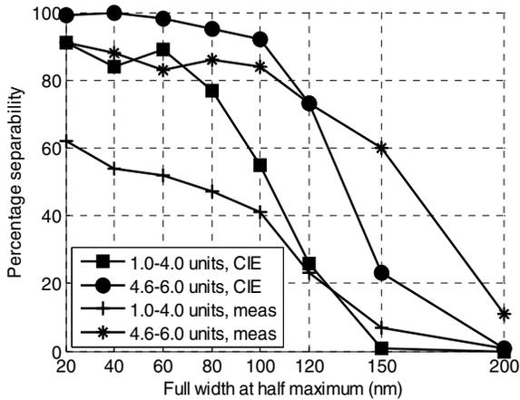
**Figure 8.** Results of the optimised sensors with 10-bits quantisation showing the effect of changing the illuminant on the separability results from Munsell colours.
