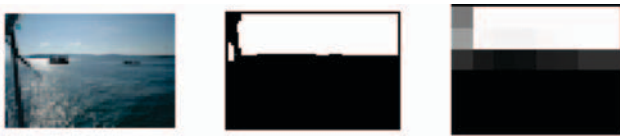
Figure 1. Left: an image from our database with a blue sky region; middle: a binary representation of the sky region’s coverage in the original image size; right: the downsampling of the binary image to 6 \times 8 pixels which is used to perform PCA. The grayscale values represent the relative coverage of the region at a given location: from 0% (black) to 100% (white)
