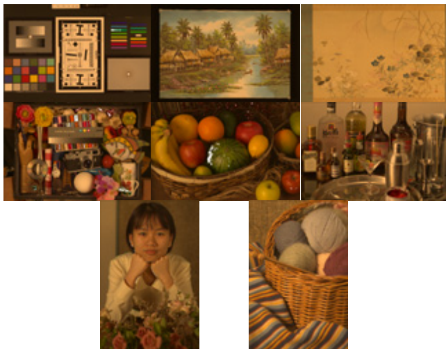
Figure 7. LabRGB encoding/decoding images P1 through P8. The pictures are for encoding/decoding using illuminant BBR4K observed by illuminant A. More than 2 \Delta E_{ab} are indicated as white color.
