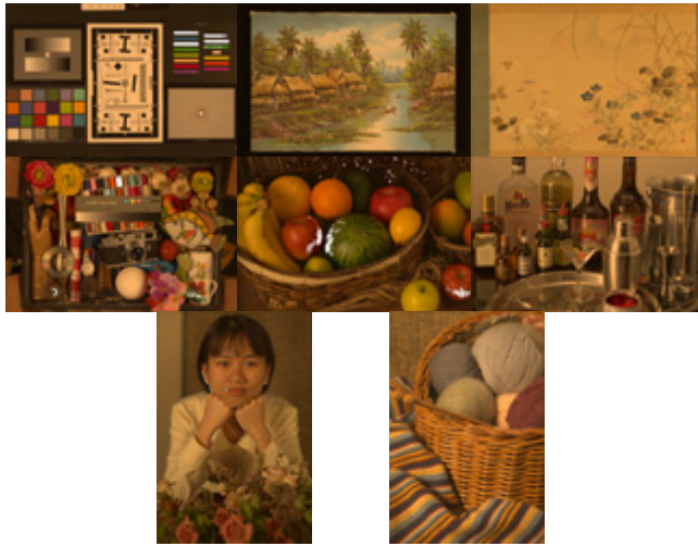
Figure 6. LabRGB encoding/decoding images P1 through P8. The pictures are for encoding/decoding using illuminant D50 observed by illuminant A. More than 2 \Delta E_{ab} are indicated as white color.
