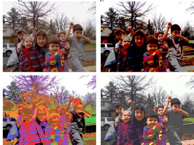
Fig. 5. Original 24 bit RGB image in upper left reduced to 27 colors using uniform device quantization in the upper right. The lower left is the original reduced to 11 color names using the algorithm of Lin et al and the lower right is the image reduced to 27 color names using lexical quantization described in this paper.
