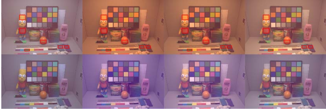
Figure 4. Row 1 shows uncorrected images and row 2 shows the corresponding corrected images. Illuminants are, from left to right, D65, A, TL83, and TL84. The red rectangles indicate the reference elements used to white balance the images. The images are rendered to sRGB using a white point preserving transform [4].
