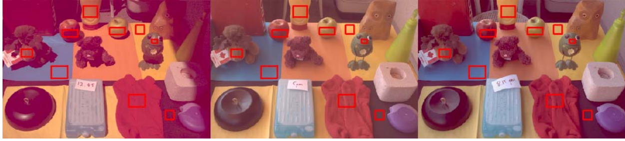
Figure 6. This figure shows uncorrected images. The red rectangles indicate the reference elements used to retrieve the illuminants, shown in Fig 5. The images are rendered to sRGB using a white point preserving transform [4].
