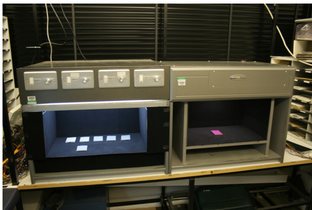
Figure 3 Two viewing booths for visual colour differences assessment.
