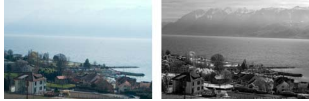
Figure 1. On the left, a conventional RGB image. On the right, a near-IR capture of the same scene. The haze has disappeared, revealing a sharper, cleaner, picture.
