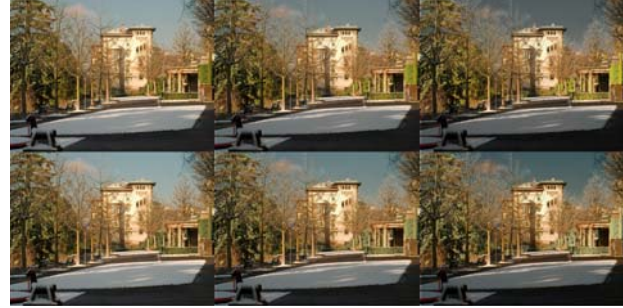
Figure 10. Top row: HSV-based rendering by blending the channels. From left to right, images where the V channel is composed of 25%, 50%, and 75% of the near-IR channel. The rest being provided by the original V channel. Bottom row: the same percentages applied to the Y channel of the YCbCr image.
