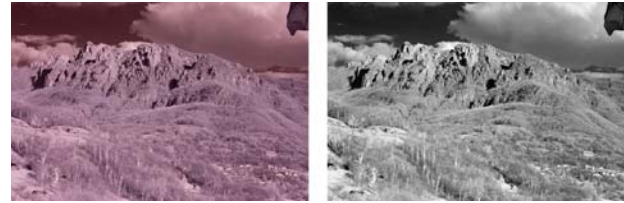
Figure 5. Near-IR image with automatic (left) and custom (right) white balance. The properly white balanced image is, straight out of the camera, effectively a grayscale image despite the presence of the CFA in front of the sensor.
