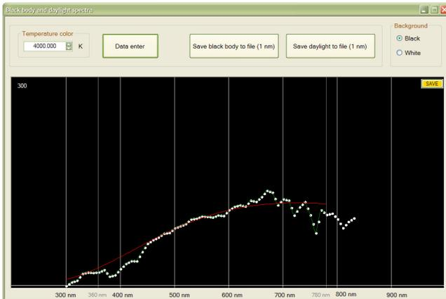
Figure 5. Blackbody and daylight spectra. Graphics given a color temperature of 4000 kelvin.
