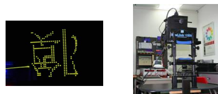
Figure 12. Left: Sample image of saccadic display captured by a camera with extended exposure. Right: A video-based eye tracker used to record and capture eye movements.
