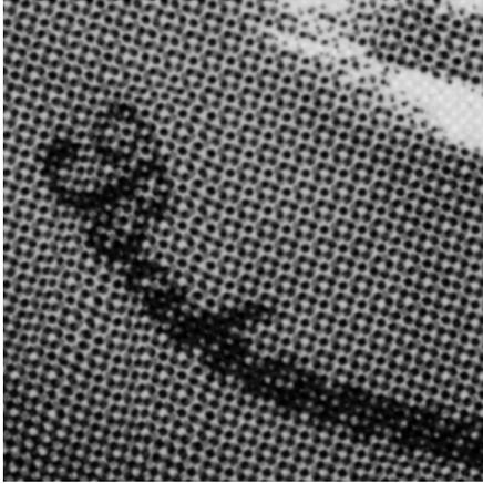
**Figure 2.** Enlarged view of a region from the scanned G channel image  $I_G^s(x,y)$  showing the coupling between the halftone structures from M separation and C and Y separations.
