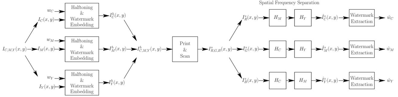
Figure 1. Overview of clustered-dot color halftone watermark embedding by exploiting spatial frequency separation principle.
