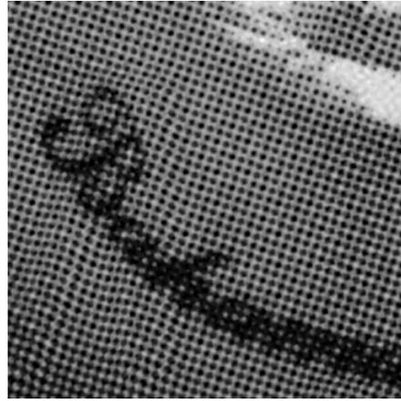
**Figure 4.** Enlarged view of the region shown in Fig. 2 after cleaning out the frequencies corresponding to C and Y halftone screens.
