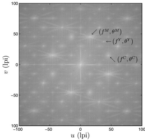
**Figure 3.** Enlarged view of the log-magnitude Fourier spectrum of  $I_G^s(x,y)$ . For illustration purposes, the frequencies of the constituent halftone separations are indicated by arrow and text labels.
