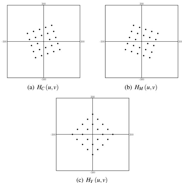
Figure 6. Spatial frequency separating filters for estimating the C, M, and Y halftone separations from the scanned R, G, and B channel images.
