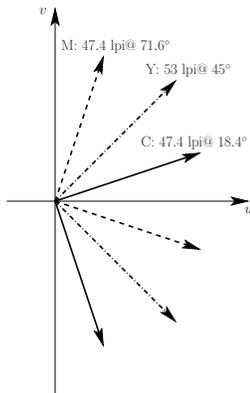
Figure 5. Frequency vectors for C, M, and Y halftone screens.
