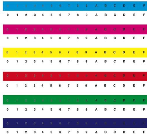
Fig. 5 Visual luminance-matching experimental target. The task of an observer was to pick the numeral that was the most difficult to read against the background.
