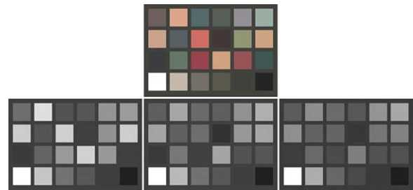
Figure 6 (top) shows the digital color image selected by observer matching for narrowband 546 and 625 nm light. Figure 6 (bottom) show the digital R, G, B separation images.
