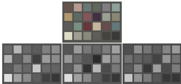
Figure 5 (top) shows the digital color image selected by observer matching session for 1 candle at 4 meters indirect light. Figure 5 (bottom) show the digital R, G, B separation images used in making the color image on the display.
