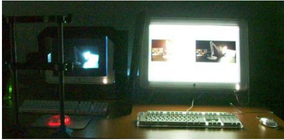
Figure 8. Experimental setup for tone-mapping algorithm evaluation using HDR display
