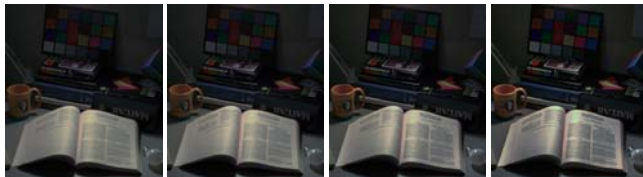
(a) 10 cd/m 2 (b) 100 cd/m 2 (c) 1,000 cd/m 2 (d) 10,000 cd/m 2 Figure 9. Predictions of the Hunt effect and the Stevens effect.
