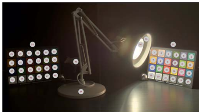
Figure 3. Locations and numerical denotations of the scene elements measured and scaled in the Luxo Double Checker scene.
