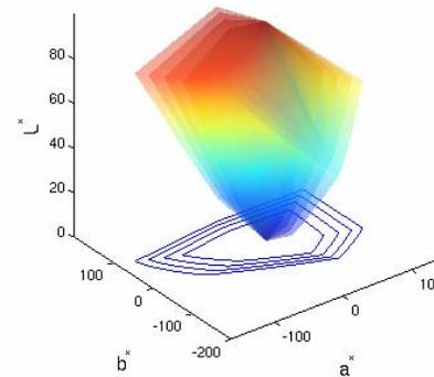
Figure 2: Actual perceptual gamut of the display in CIELAB with successive color gamut volume reductions of 1.0, 0.8, 0.6, and 0.4 times the full, extended gamut of the display for the MCSL experiment
