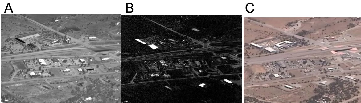
Figure 2: Registered multimodal imagery of an aerial scene where panel A is an LWIR thermal image and panel B is a polarimetric image of the same scene acquired at the same time. These images would be largely invariant to time-of-day because the scene is sensed in the LWIR. Panel C is a Visible three-color image of the same scene. Our aim is to create a mapping strategy that takes data like those in panels A and B without 3-band visible information and renders them to look like panel C using segmentation, database information, and false illumination.
