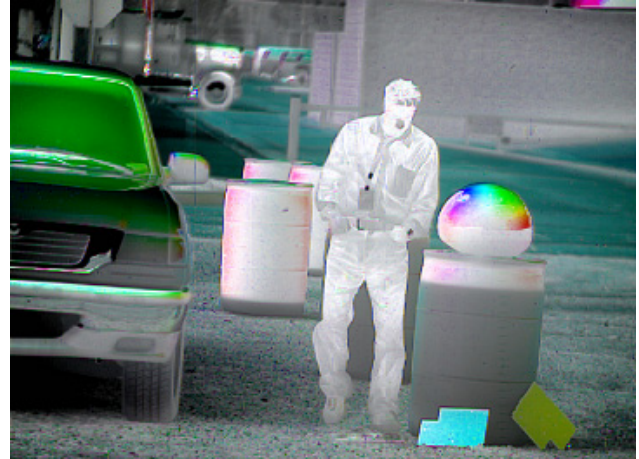
Figure 1: Image showing application of our developed thermal/polarimetric color fusion strategy. Our fusion scheme has been run in software in real-time on a PC, and can be easily incorporated into a real-time DSP platform. In the color scheme color saturation is the degree of polarization, hue corresponds to object shape and orientation and the infrared image is mapped to value.
