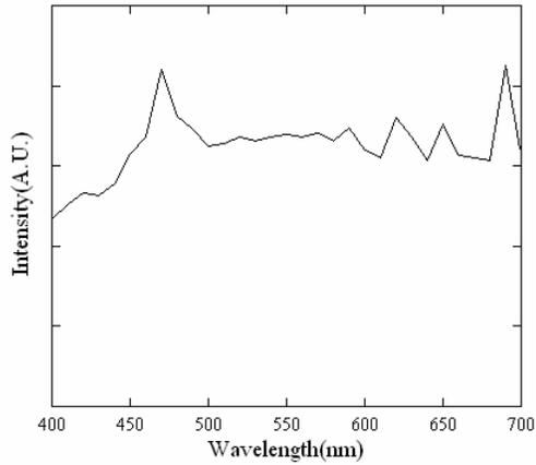
**Figure 2. Spectral power distribution of the illuminant used image acquisition.**
