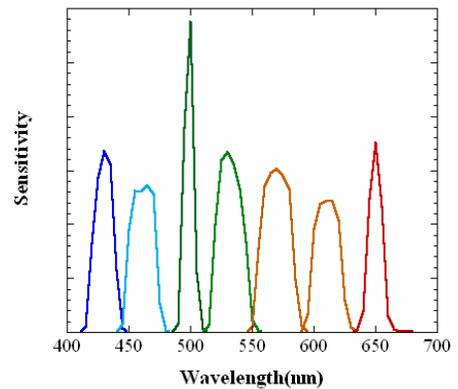
**Figure 1. Spectral sensitivities of the multispectral camera used in this experiment.**
