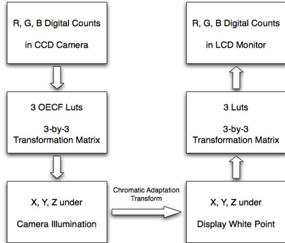
Figure 9. The flowchart of color management for image rendering
