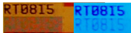
Figure 4. Fluorescence watermark example seen under normal light (left) and UV light (right). The alpha-numeric sequence seen in the upper portion has been duplicated as a watermark in the lower portion, and should be revealed in the right-hand image.
