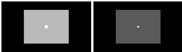
Figure 8. Generated images for measurements. Left: Background: 50% of \Psi_{max} , Specular highlight size: 1.1 degree. Right: Background: 10% of \Psi_{max} , Specular highlight size: 0.55 degree.
