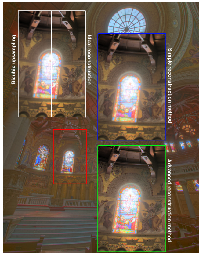
Figure 6. An image of the Stanford Memorial Church mapped with a bilateral filter, and recovered using the simple and advanced methods from a 4x downsampled HDR version. (Image courtesy Chris Cox of Adobe Systems.)
