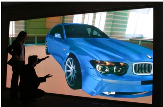
Figure 1. High resolution stereoscopic tiled display with 48 beamers (courtesy of Fraunhofer IGD).
