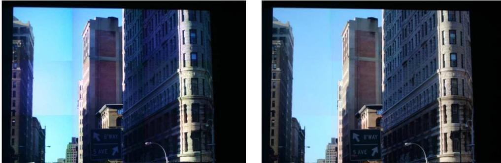
**Figure 7.** Example of corrected image: before correction (left), after intra-projector and inter-projector calibration (right).
