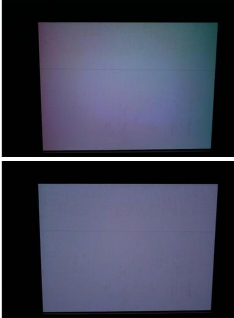
**Figure 4.** A projector before (top) and after (bottom) intra-projector correction.
