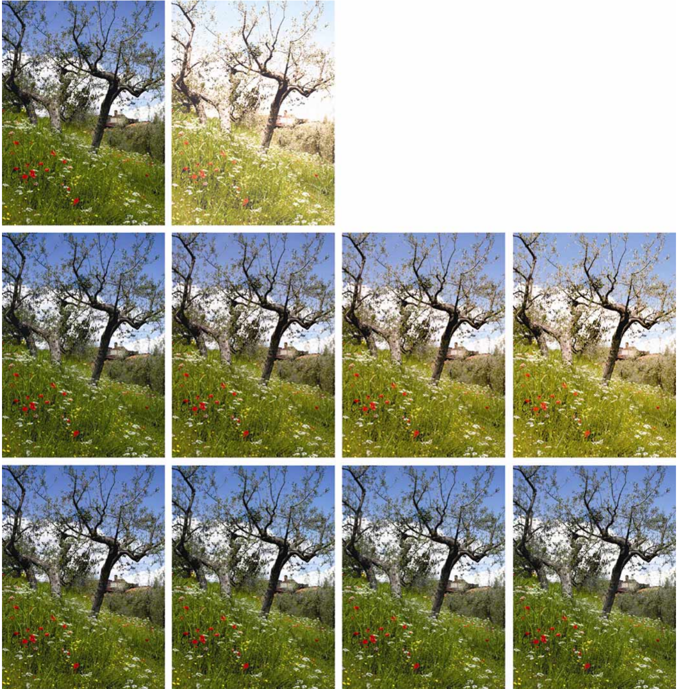
Figure 4. Color simulations (generated for a SWOP CMYK output device) of how an image will look like after 0 years (column 1), after 30 years (column 2), after 60 years (column 3) and after 90 years (column 4) for an image printed on inkjet printer #1, paper A (row 1), inkjet printer #1, paper B (row 2), and inkjet printer #2, paper C (row3).
