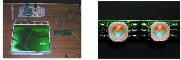
Figure 13. Exposed side-lit LED backlights on top and bottom with the driver board (left). An LED chip consists of one red, two green, and one blue LEDs (right), whose spectra are spikier than CCFL's (top).
