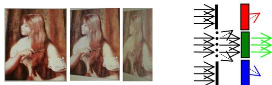
Figure 2. Left: Luminance/contrast degrades and color shifts as viewing direction increases from 0° to 30° and 60° on a 19" TFT-LCD. Right: The backlight of a green subpixel leaks into its adjacent red and blue color filter and causes color shift.
