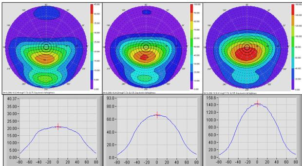
**Figure 3.** Luminance vs. viewing direction measured by a *ConoScope* for on graylevel 75, 135, and 195 (from left to right). The upper and lower charts show the luminance distributions in a hemisphere and on the 9-to-3-o'clock plane, respectively.
