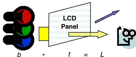
Figure 1. Backlight, transmittance, luminance, and light leakage.
