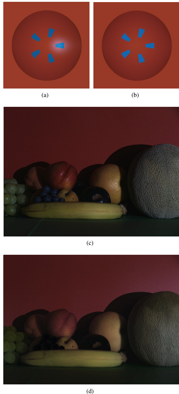
Figure 3. Experimental results. Figure (a) shows a synthetic image of a sphere made of two different materials. Figure (b) shows the specular-free image obtained by analyzing, for any given pixel location, all observed colors. All the small patches of this image have the same body color. Figure (c) shows an image taken from the specular subset of the Simon Fraser University dataset. Figure (d) shows the recovered specular-free image. Note that surfaces in this image do not look as shiny as the surfaces of the image in Figure (c).
