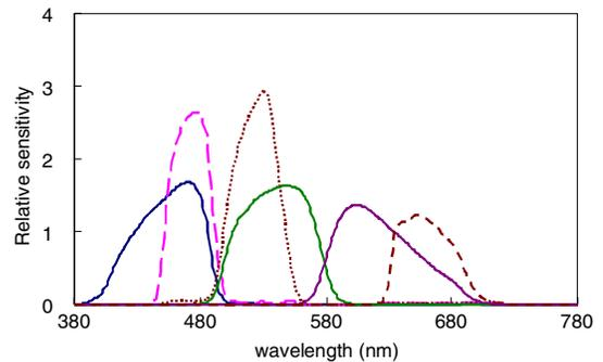
Figure 6 The spectral sensitivity of 6-band multispectral camera. Dashed and solid curves represent narrow bands and unmodified wide bands, respectively.
