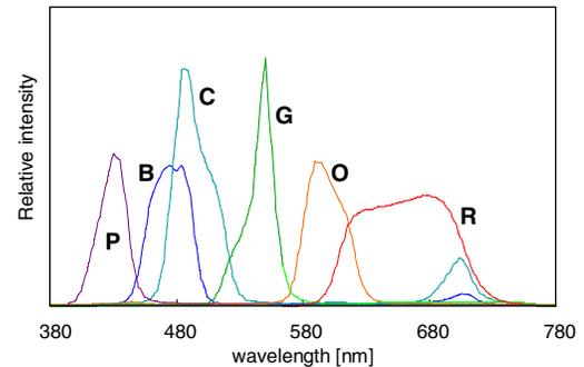
Figure 7 Spectral radiances of primary colors in 6-primary RPD. Primaries P, C, R, and B, G, O are generated by projector #1 and #2, respectively.
