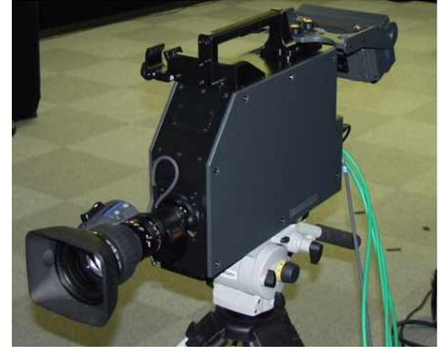
Figure 5 6-band HDTV video camera used in this experiment.
