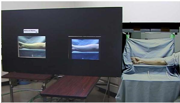
**Figure 10** Setup for the direct comparison of the real skin and the reproduced images by NV-6B (left) and C-3B (center) systems.
