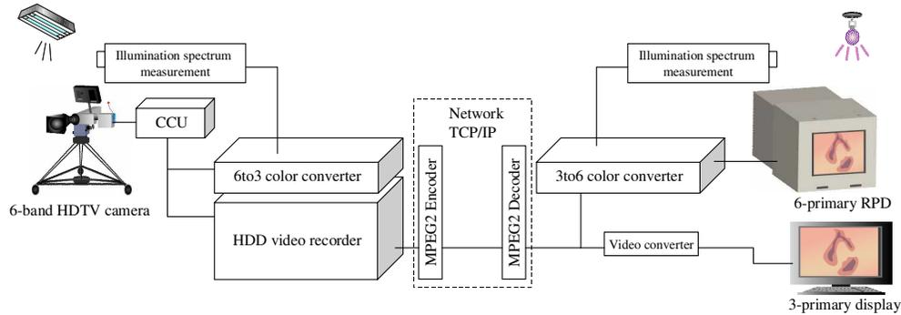
**Figure 1** Schematic diagram of prototype 6-band multispectral video system. CCU: Camera control unit, RPD: Rear-projection display.
