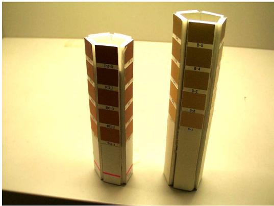
Figure 4 Skin color chips on pentagonal cylinders used in the experiment.
