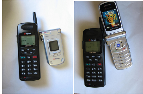
Figure 1. Samsung SCH1000 (1997) and Samsung a940 (2005). The former has a monochrome 3-line 12 character LCD (5 × 7 pixels for each character) voice only phone while the later has a 176 × 220 pixels 262K color full graphics TFT display, an external 96 × 96 pixels 65K color TFT LCD with 2Mp camera and 2x optical zoom
