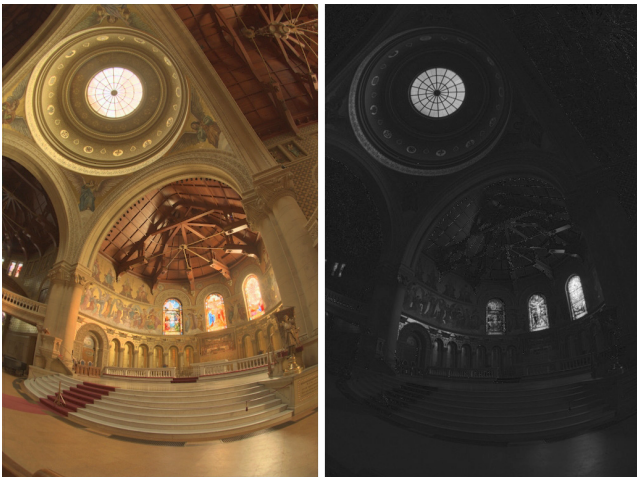
Figure 3. Memorial Church shown tone-mapped with Reinhard's global operator (left) along with the log-encoded ratio image needed for HDR recovery (right).
