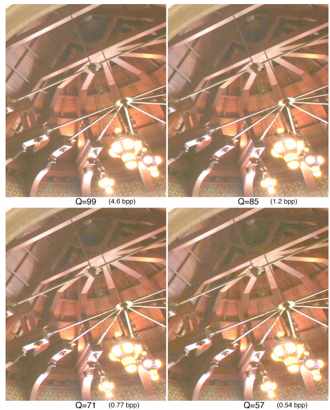
Figure 7. Quality of recovered image at different compression settings using subband pre-correction method and Reinhard's global TMO (bits/pixel in parentheses).
