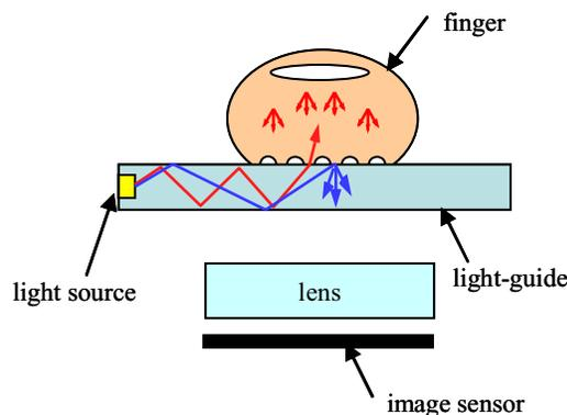
Figure 2. A sensor based on scattered-light detection.
