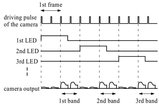
Figure 7. Driving sequence for the multi-spectral imaging
