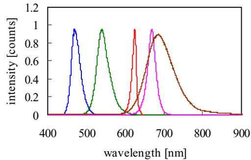
Figure 6. The emission spectra of the five LEDs used in this experiment
