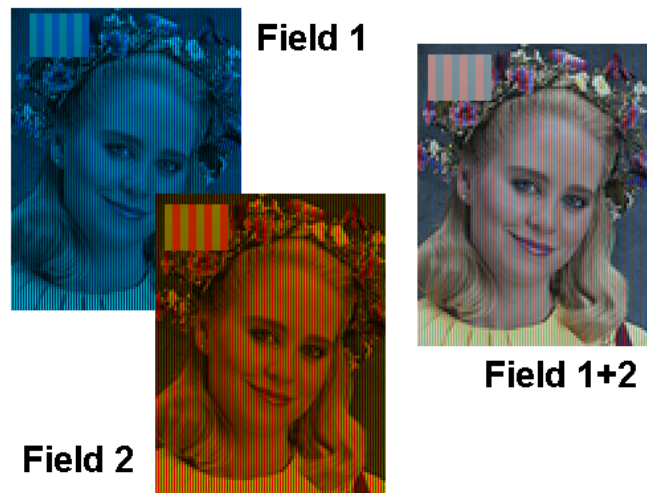
Figure 6. Illustration of the two fields in the case of an actual image of a girls face and the resulting image as seen by the eye when presented at a refresh rate of 120 Hz. The left corner shows a zoomed image of the forehead. One can clearly see the striped pattern and the difference in the color of the pattern in each field and the resulting field.
