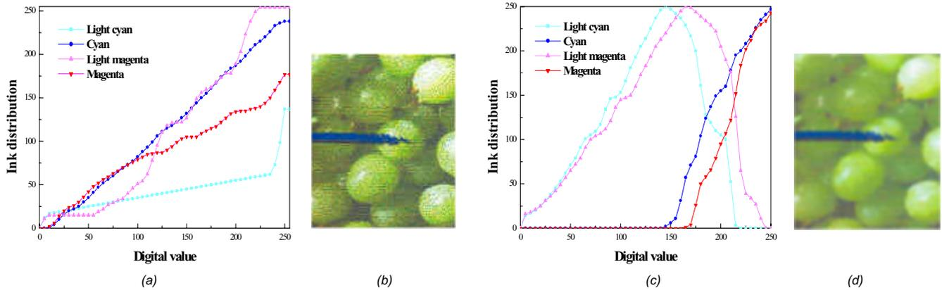
Figure 1. Conventional six color separations; (a) Photo-ink separation pass of the six color separation using the color difference (b) Result of the six color separation using the color difference (c) Photo-ink separation pass of the six color separation using the lightness and subjective granularity (d) Result of the six color separation using the lightness and subjective granularity
