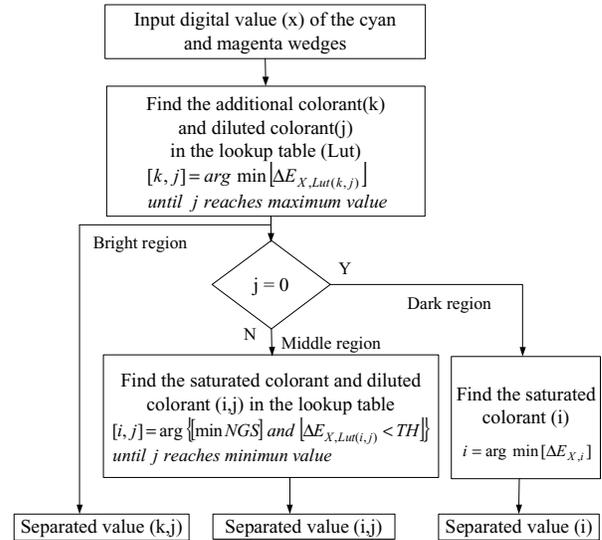
Figure 3. Block-diagram to construct three lookup tables for proposed six color separations
