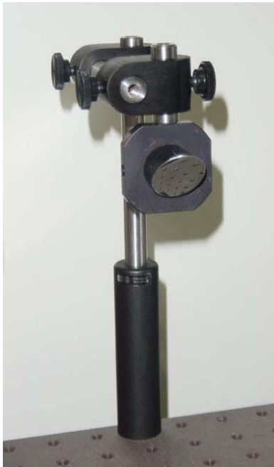
Figure 7. Off-axis concave parabolic mirror used in prototype.
