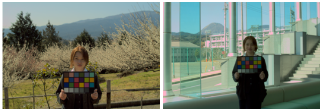
Figure 6. Artifacts in the rendering images (Left image is rendered by sigmoid transform, the right image is rendered by photographic reproduction)
