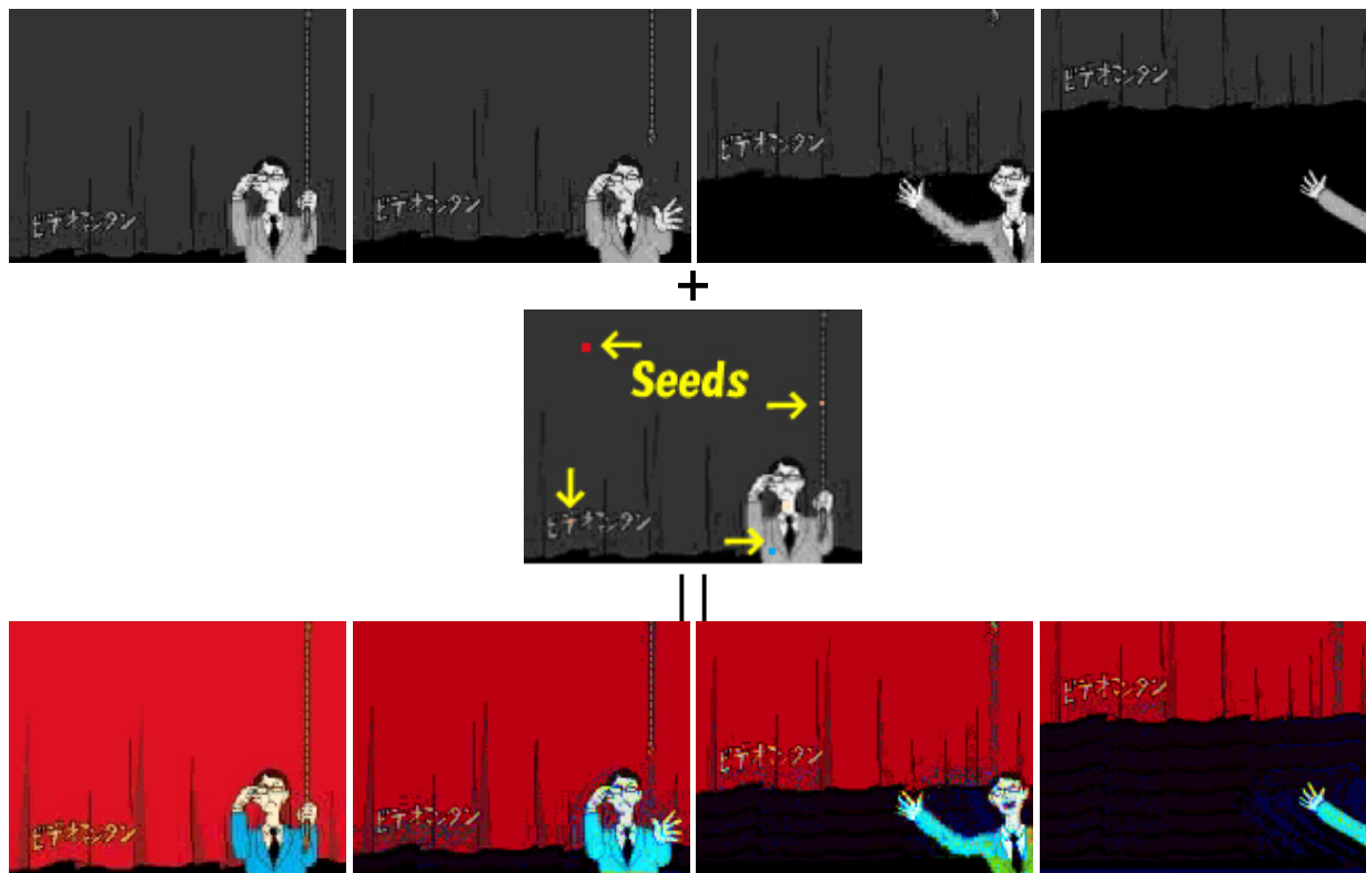
Figure 1. A sequence of monochrome images (upper) is colorized (lower) by giving a few color seeds to the first frame (middle).
