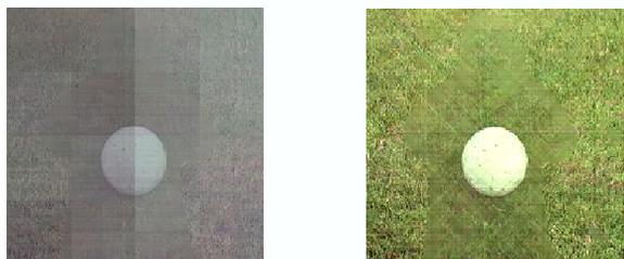
Figure 7: Example of recovering a shadow-free image. The path used are a horizontal raster and a diagonal raster (again, with all rotations i.e. 16 paths). Top left: Original Image; Top right: the shadow mask; Bottom left: the image obtained after reintegration; bottom right: the image obtained after color rescaling
