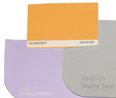
Figure 3 is a photograph of the three papers used in these experiments. They are most closely matched to the Munsell Book in tungsten light by N 7.5, 2.5Y7.5/10, and 2.5P8/6.
