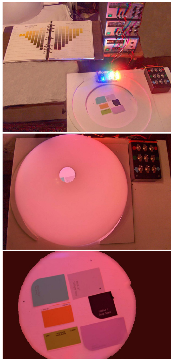
Figure 1 (Top) shows the experimental apparatus. A collection of papers are placed on a white background. Adjacent to the papers is an array of 12 LEDs - four 625nm, four 530nm and four 455nm. The photograph shows the 421 configuration, meaning that all four 625 LEDs are on, two 530 are on and one 455 is on. The relative intensities of long-, middle and short wave illumination is controlled by the number of LED emitters. The black box on the right contains the on/off switches. The constant voltage power supplies for LEDs are in the upper right. The Munsell Book for color matching is shown in the upper left.
