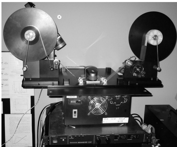
The autoadvancing Eye-One spectrophotometer
