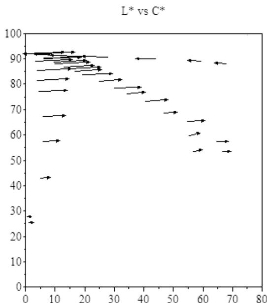
Figure 5. UV excluded to UV included  $L^*$  vs.  $C^*$  difference vector plots. Data shown for CMYK ramps of device CA, substrate EPS.
