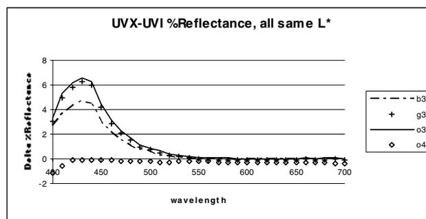
Figure 1. UV included – UV excluded percent spectral reflectance of four offset printing substrates with UVI and UVX  $L^* = 93$ .
