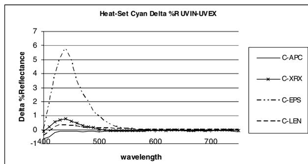
Figure 4. UV included – UV excluded percent spectral reflectance of heat-set cyan on different substrates.
