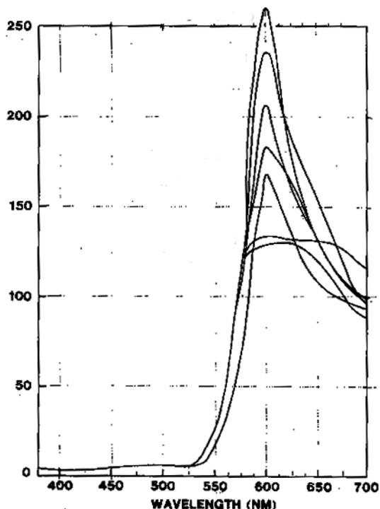
Figure 2. Percent total spectral radiance factor of daylight-fluorescent DayGlo® ArcYellow ink measured on seven commercial instruments containing sources of various CCT.<sup>6</sup>
