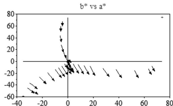
Figure 6. UV excluded to UV included  $b^*$  vs.  $a^*$  difference vector plots. Data shown for CMYK ramps of device CA, substrate EPS.
