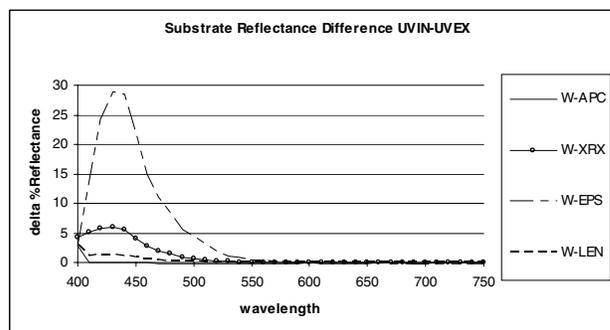
Figure 3. UV included – UV excluded percent spectral reflectance of experimental substrates.
